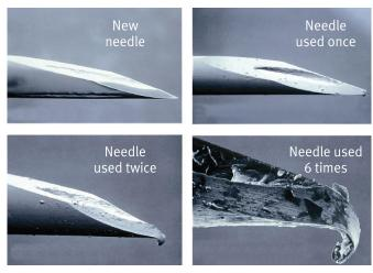
Figure 5. Needle reuse damages the tip of the needle.
